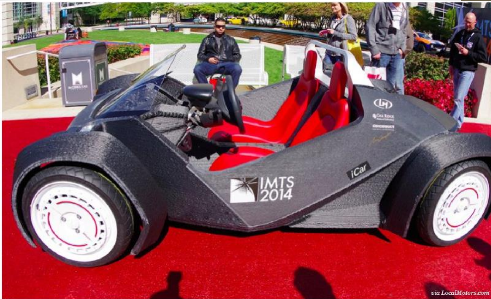
The Strati, the world's first 3D printed electric car.
